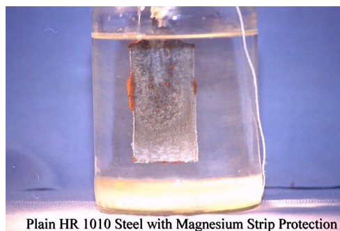
Plain HR 1010 Steel with Magnesium Strip Protection
