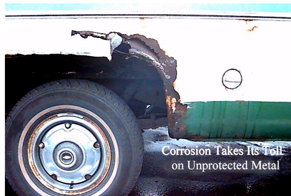
Figure 1. An older vehicle shows the effects of corrosion
