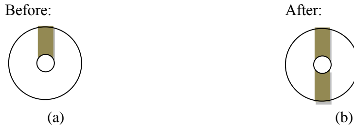
Figure 3 - Design improvement of the metal contacts (top view) for Lighted Ball Point Pen [10]
