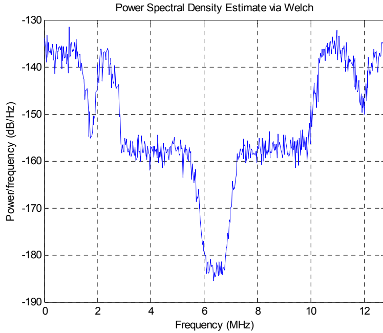
Figure 9: Baseband Spectrum of a Digital TV Station
