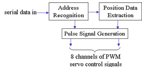
Figure 5: SSC Block Diagram
