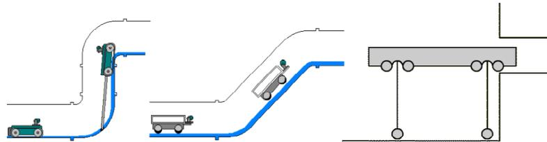
Figure 11: Three Options for Negotiating the 18 Inch Elevation change
