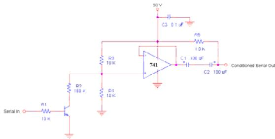
Figure 7: Telephone Line Simulation Circuit
