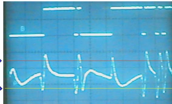
Figure 9: Distorted and Reconstructed Serial Data Pulses
