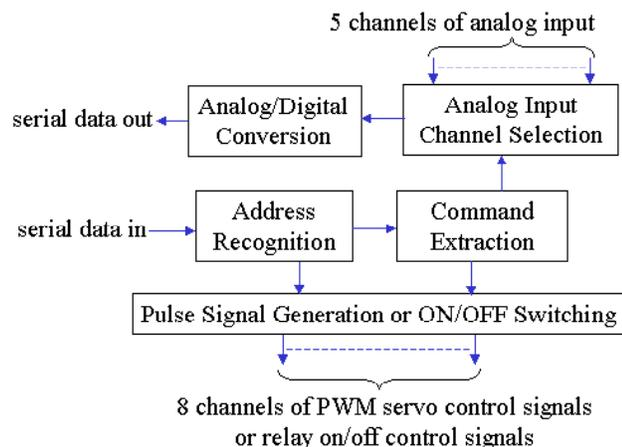
Figure 15: Block Diagram of the SV203 Controller
