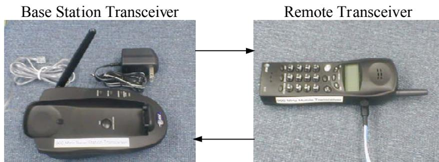
Figure 1: 900 MHz Communication Link
