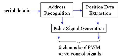
Figure 5: SSC Block Diagram
