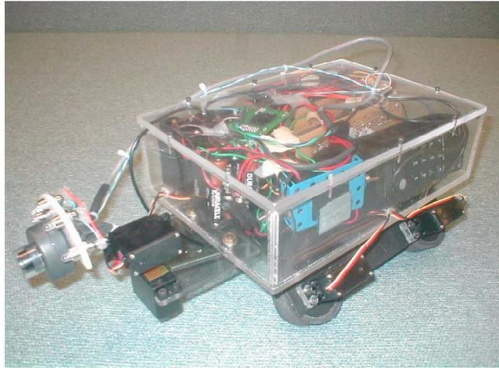
Figure 13: The Sewer Navigating, Wireless Robot
