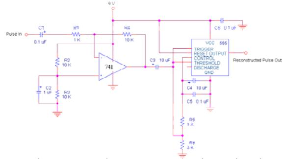
Figure 8: Pulse Reconstruction Circuit
