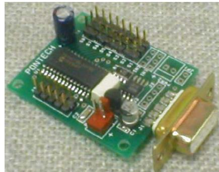
device we would consider using next time is a SV203 Servo Motor Controller,<sup>7,8</sup> as depicted in Figures 14 and 15.
