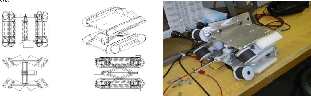
Figure 12: An Expandable, Tracked Robot
