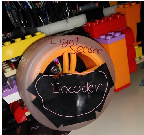
Figure 6: Custom encoder developed by the team to measure position
