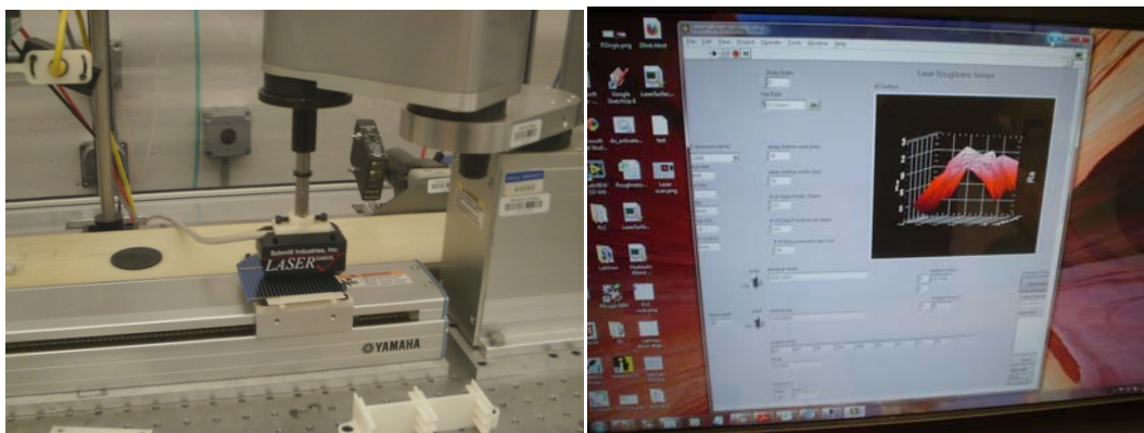
Figure 7: LabVIEW interface for surface profiling
