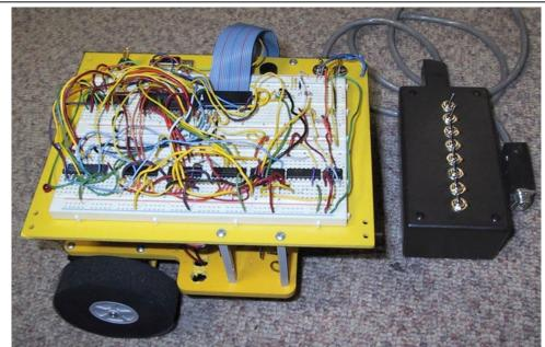
Figure 1: The custom robot base used at VMI. Students add soldered PC boards that they assemble (e.g. an H-bridge motor controller and contact sensors) to the frame, and build the digital logic on the supplied solderless protoboard. The teaching pendent used for programming is shown to the right.
