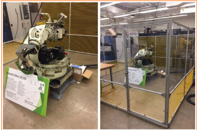
Figure 2. Robot assembled in the protective cage
