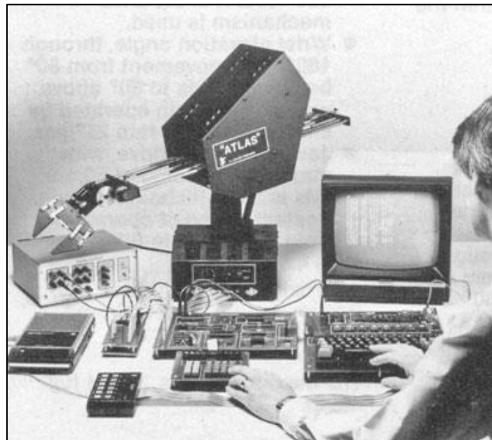
Figure 1: L.J. Electronics ATLAS Robot controlled via an EMMA Microcomputer [6]
