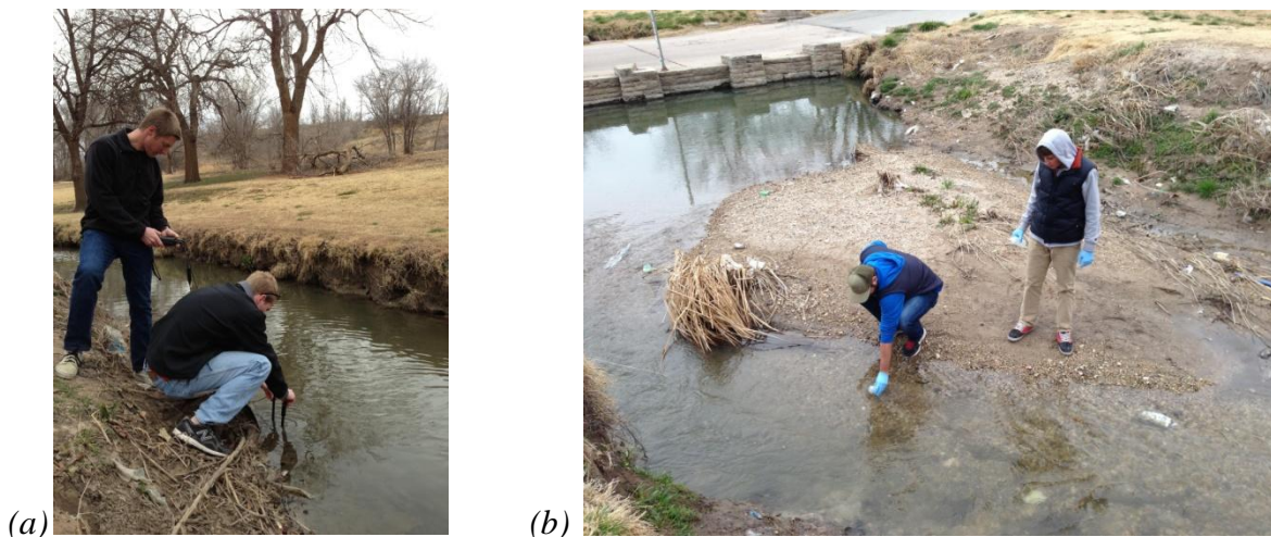
Figures. (a) Students using pH, TDS, and DO probes to take real time field measurements. (b) Students collecting field samples to be processed later in the lab.
