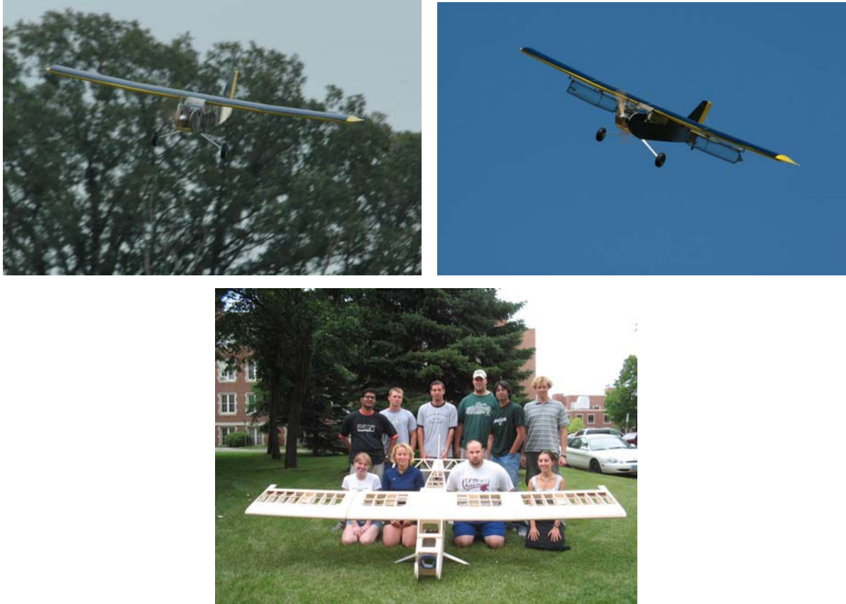
Figure 5. Upper Left: Albatross Unmanned Aerial Vehicle in flight (3-meter wingspan, capable of carrying payloads in excess of 4-kg). Upper Right: Albatross UAV with the BugHunter payload installed, used for controlled mosquito catching above the ground. Bottom: 2004 NSF REU Site participants next to the R/C airplane during its construction.
