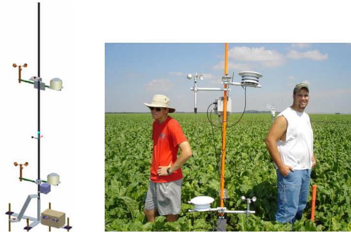
Figure 6. Left: CAD representation of the wireless sensor weather station. Right: Undergraduate engineering student weather station designers in a local sugar beet field. From this figure, you are able to get a sense of the height of the sugar beet leaf canopy later in the growing season. The lower anemometer indicated a much lower wind speed near the canopy than the upper-level anemometer, which gave the REU Site participants an intuitive understanding of why the differential measurements were needed.
