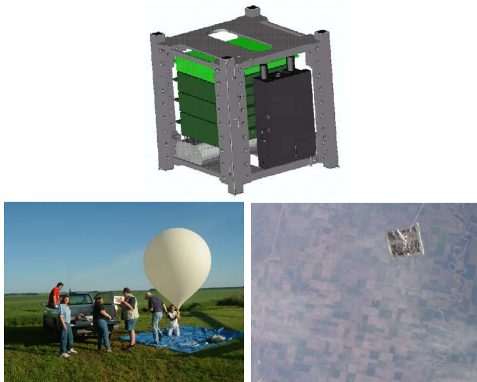
Figure 4. Top: CAD representation of CTAAP – CubeSat To Accept Any Payload. Bottom Left: CubeSat weather balloon launch on a perfect summer day in 2003! Bottom Right: In-flight digital picture taken at 96,400 feet, with a radar reflector suspended below the satellite. The CubeSat was recovered, intact and operational, by the REU Site participants.
