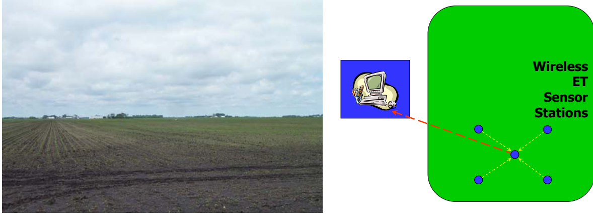
Figure 7. Left: Sugar beet field at the beginning of the growing season. Right: Wireless ET sensor station placement in a sugar beet field. The center ET station is capable of relaying data to a farmstead-based Web server through a long-range (i.e., 30 km) line-of-sight transceiver, while the other four ET stations are only equipped with motes for short-range (i.e., 100 m) communications.
