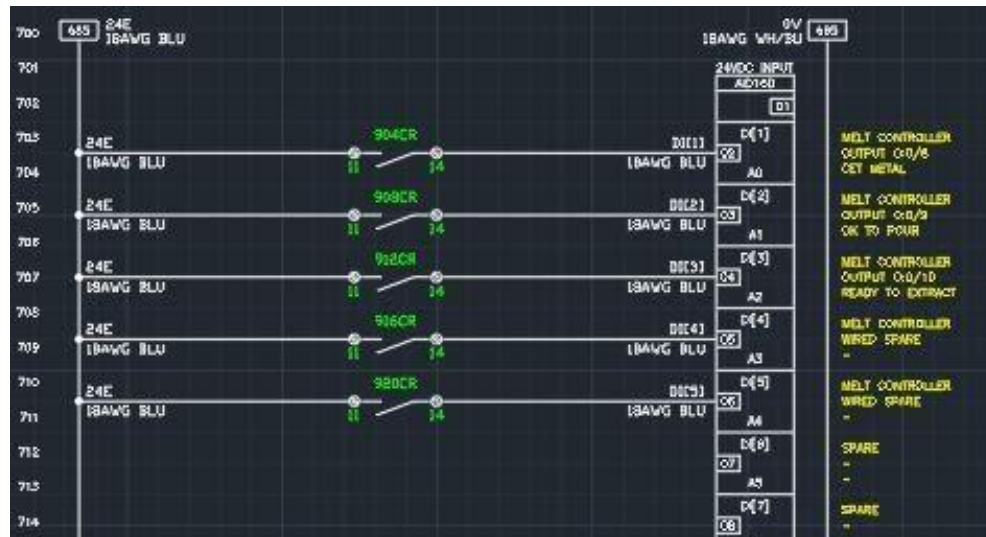
Fig. 2. The PLC input wiring diagram as provided by FANUC with the R1000-iA/80F robot. The inputs shown are used in conjunction with a melt controller for the previous application.
