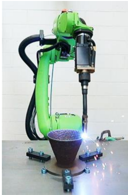
Fig. 5. A FANUC robot designed for an integrated with a Lincoln welding unit for 3-D welding projects.
