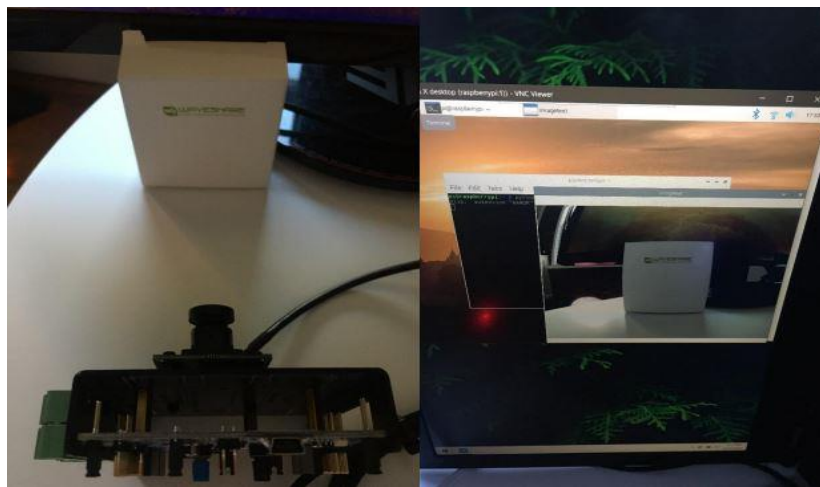
Fig. 10: Demonstration of functioning camera over the tether cable
