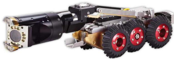
Fig. 2: Aries Industries Pathfinder TR3320 robot with infinite rotation camera [11]
