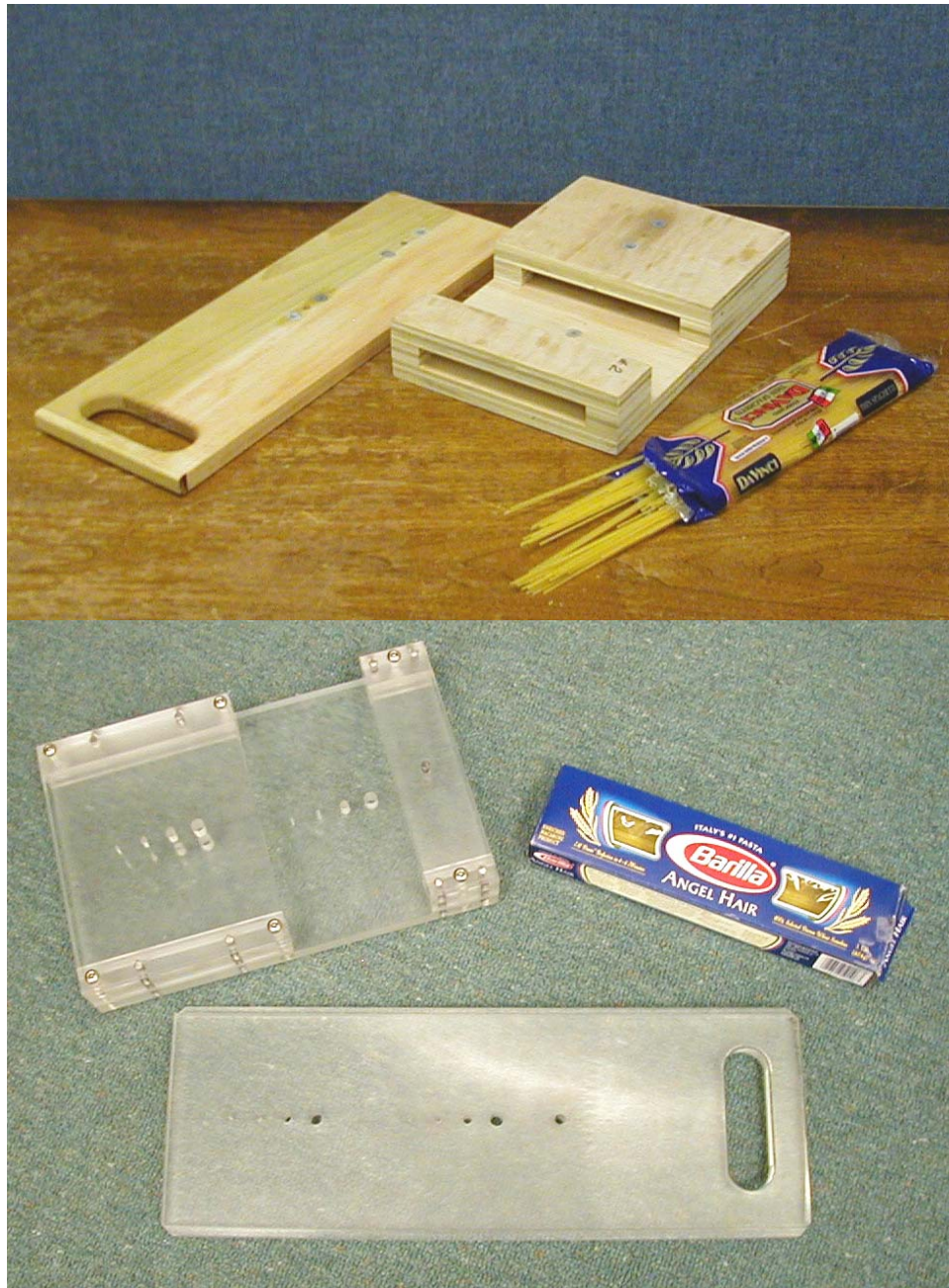
Figure 2: Shear Demonstrators. Above: Wooden, Below: Acrylic
