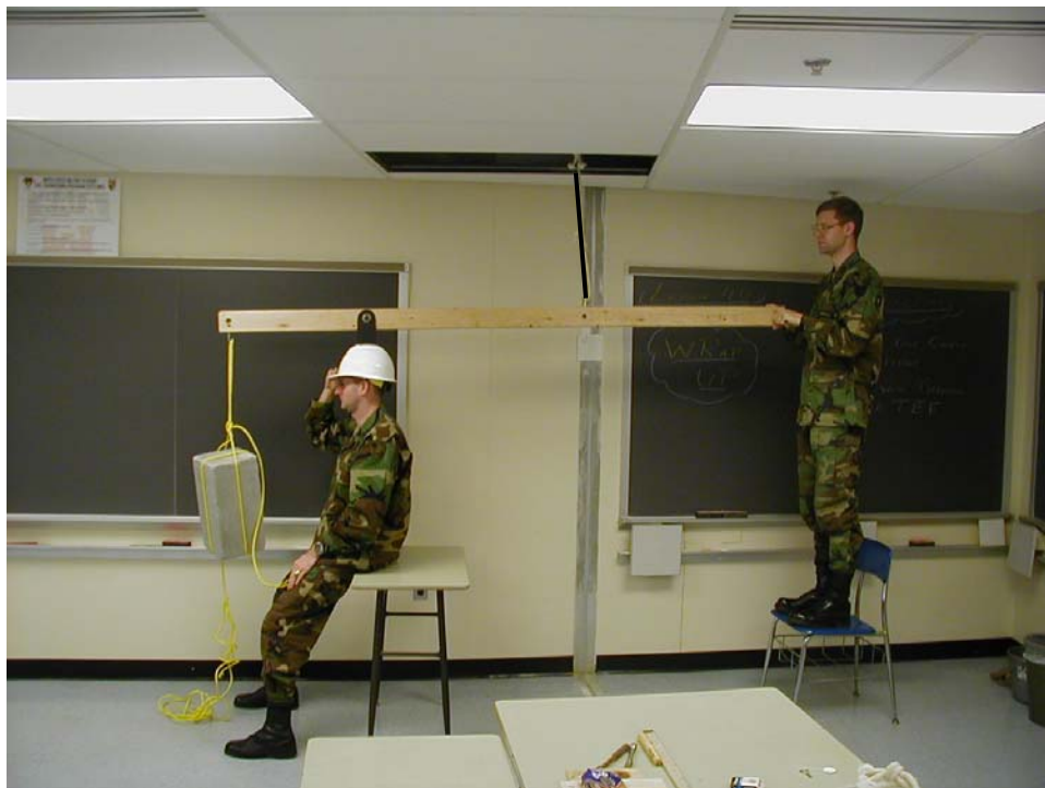
Figure 3: Demonstration of Statically Indeterminate Systems; "The Compression Cadet"
