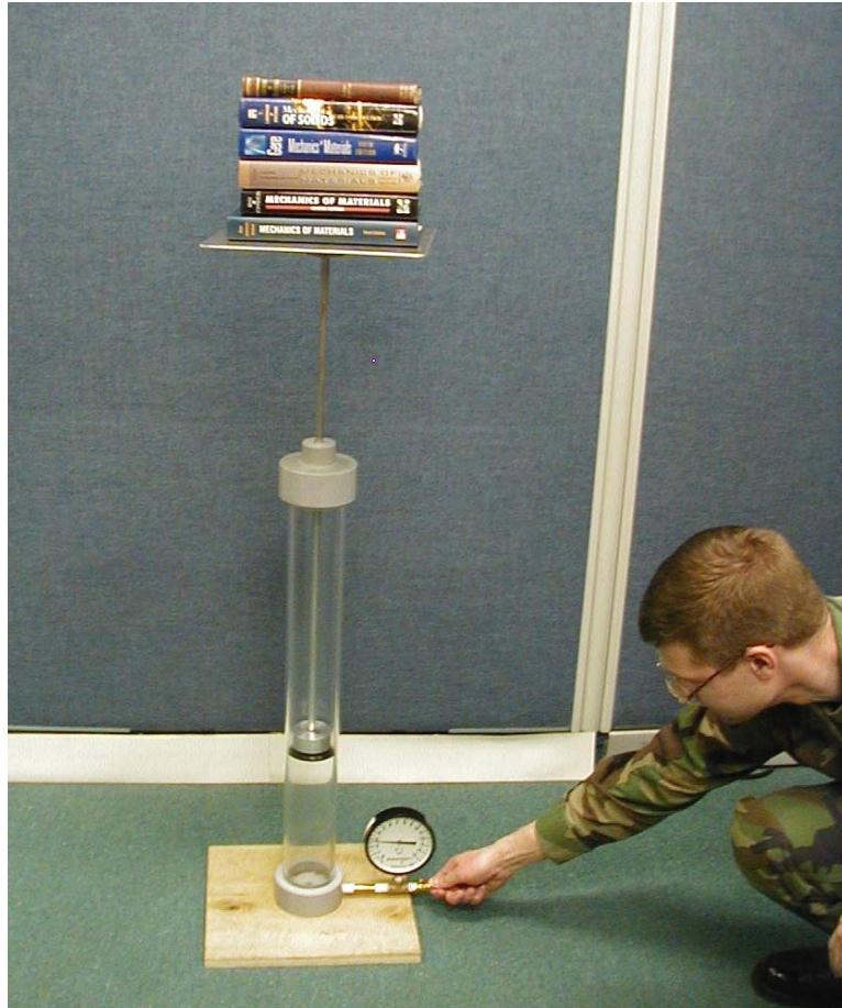
Figure 1: The Stress Demonstrator (Shown here on the ground. Recommend elevated use for student visibility)
