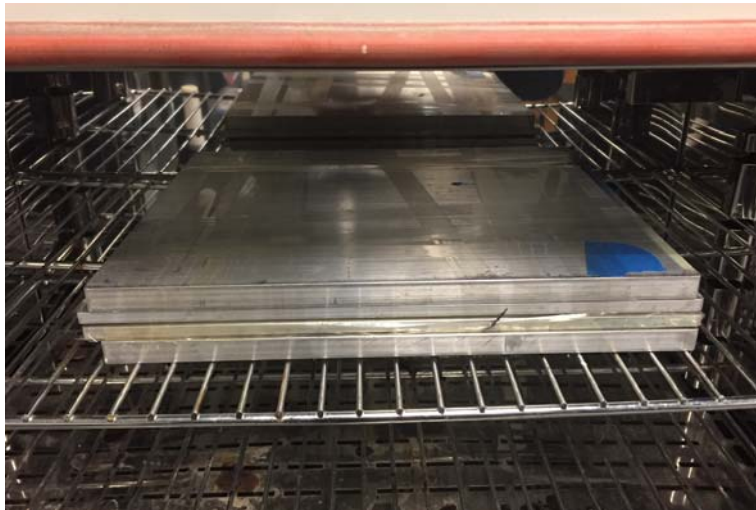
Figure 5 Specimens Between Aluminum Plates in Curing Oven.
