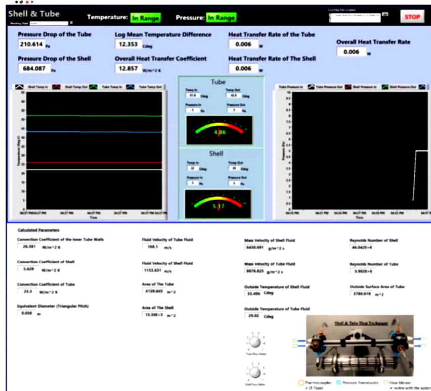
Figure 3. The current version of Shell and Tube heat exchanger interface for laboratory activity in LabVIEW™
