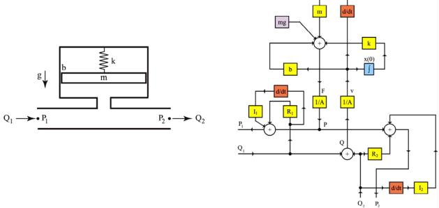
Figure 7 Accumulator and associated simulation diagram.
