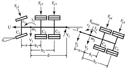
Figure 5 Conceptual sketch of the El-Gindy semi tractor-trailer.
