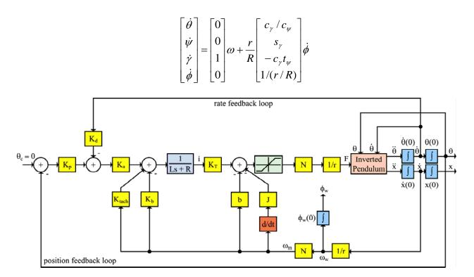
Figure 3 Simulation diagram of an inverted pendulum stabilized with proportional and derivative feedback control action.
