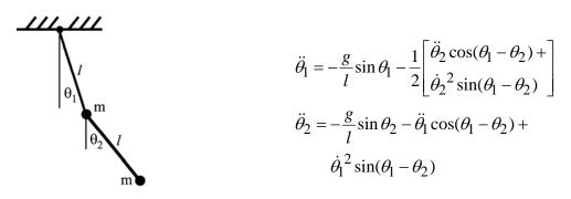
**Figure 11** The N = 2 pendulum chain approximation of a weighted string: conceptual figure and corresponding coupled ordinary differential equations (Robert Ertel).
