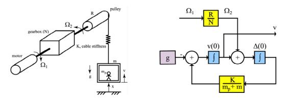
Figure 2 Conceptual sketch of an elevator system and corresponding simulation diagram.
