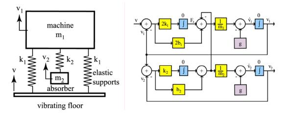
**Figure 1** Conceptual sketch of 1D vibration absorber attached to a vibrating machine and associated simulation diagram (with damping present as well).
