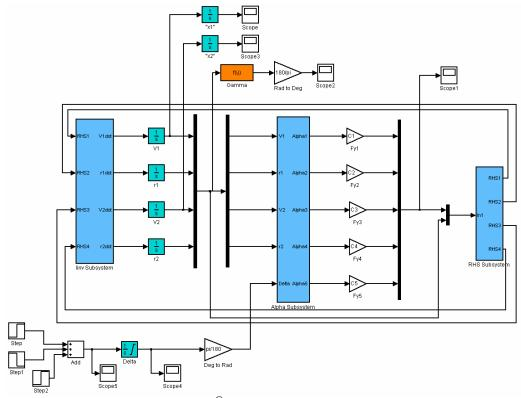
Figure 6 Top-level Simulink<sup>®</sup> model of the El-Gindy semi tractor-trailer.
