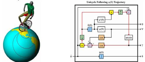
Figure 4 Unicycle on a sphere with corresponding contact point trajectory driven simulation diagram that contains an embedded algebraic loop shown in red (Hennessey, 2006a).
