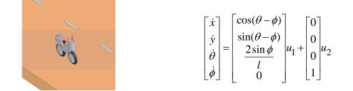
**Figure 10** The kinematic car model depicted in CAD with both front and rear wheel steering in preparation for a performing a passing maneuver on a highway and described analytically in control input form (Lina Salah and Michael Zimmerman).
