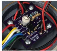
Figure 9: ThermalCAT trainer PCB board
