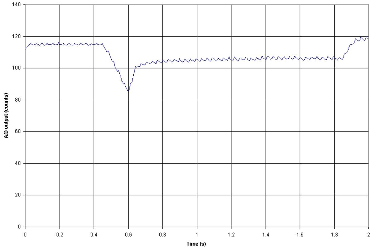
Figure 5. Raw data from an actual rocket mission using a C6-5 engine. As this is the output of an inverting amplifier, upward acceleration causes decreased output voltage. This curve was readily plotted in the field and shows that the system functioned correctly. The ripple is the switching frequency of the power supply, aliased by the sub-Nyquist sampling rate.
