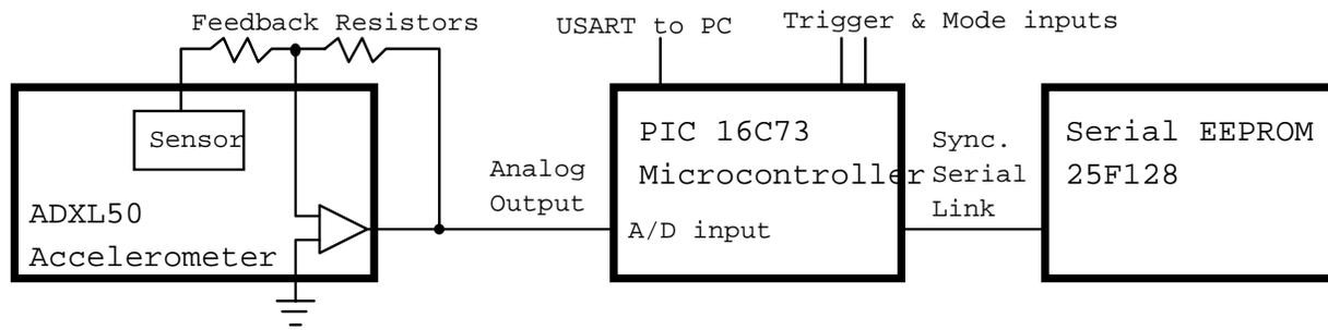
Figure 1. Block diagram of the system. The accelerometer generates a signal proportional to the acceleration the rocket sees. This signal is read by the PIC microcontroller. The PIC writes the data to the serial EEPROM, where it can reside even when powered down. After recovery, the data is sent via the USART to a laptop.
