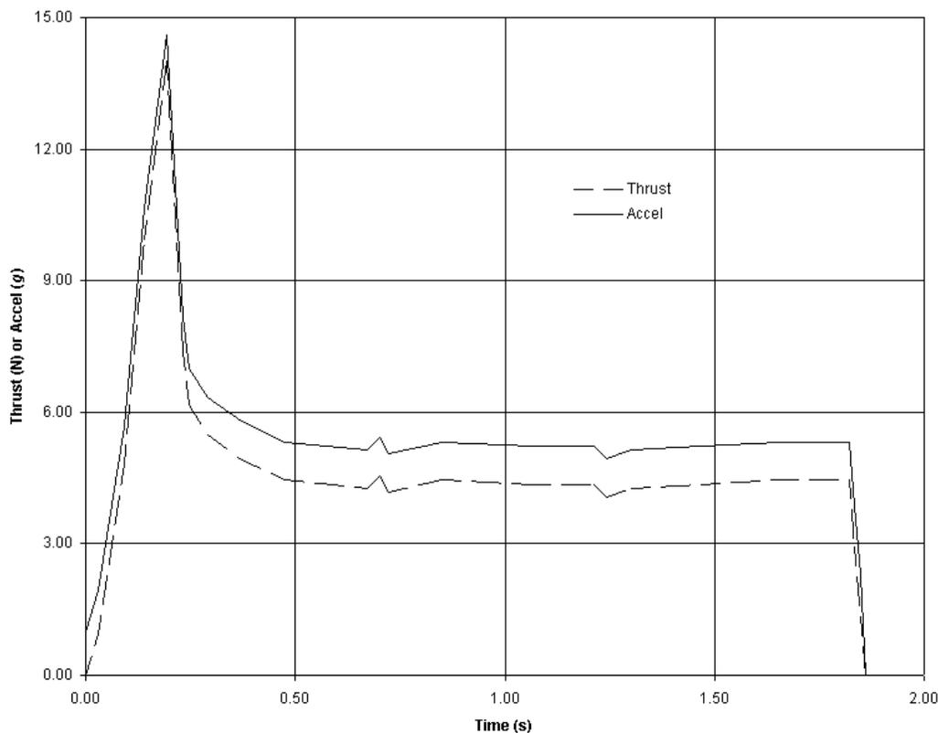
Figure 3. Predicted performance of the rocket. The thrust data was extracted from a performance curve of the Estes C6-5 engine provided by the National Association of Rocketry (NAR).<sup>2</sup> The acceleration curve for the rocket is calculated from the NAR thrust data. Note that at  $t = 0$ , the system experiences Earth's gravity, which is equivalent to a rocket accelerating upward at 1 g in free space.
