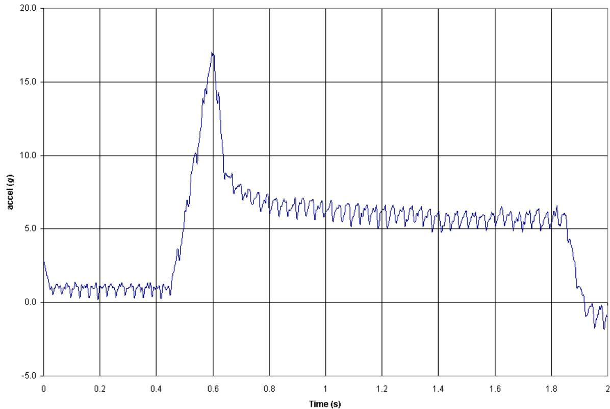
Figure 6. Processed acceleration data for the launch shown in Figure 5. The shape compares favorably to the predicted acceleration curve in Figure 3. As the measured acceleration goes negative when the engine stops firing (not zero), this calibration should be considered preliminary but sufficient for our purposes.
