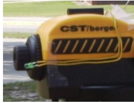
Figure 3.0 (a) Smart Rod Parallax Board Figure 3.0 (b) L.E.D Attached to Automatic Level Machine
