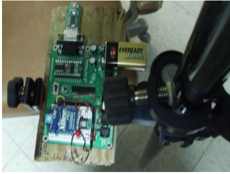
Figure 3.0 (a) Smart Rod Parallax Board Figure 3.0 (b) L.E.D Attached to Automatic Level Machine
