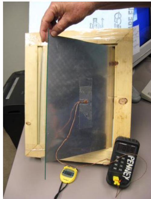
Figure 3. Experimental Setup Showing Unpainted Side with Thermocouple
