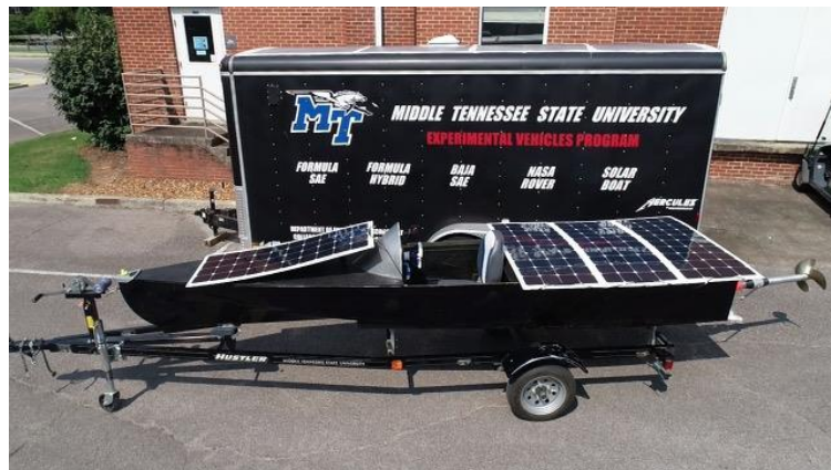
Fig. 1. Solar panel array for 2021 Solar Splash Competition.
