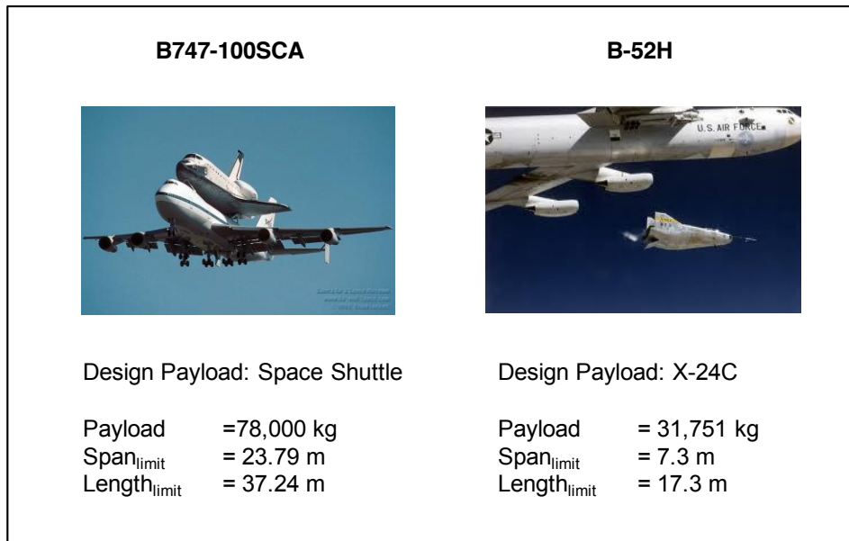
Figure 11. Summary of B747-SCA and B-52H constraints for the hypersonic demonstrator study. (Ref 15,16)
