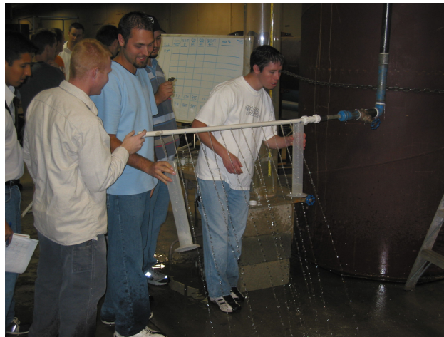
Figure 1. Students testing a lab-scale diffuser for port discharge uniformity.
