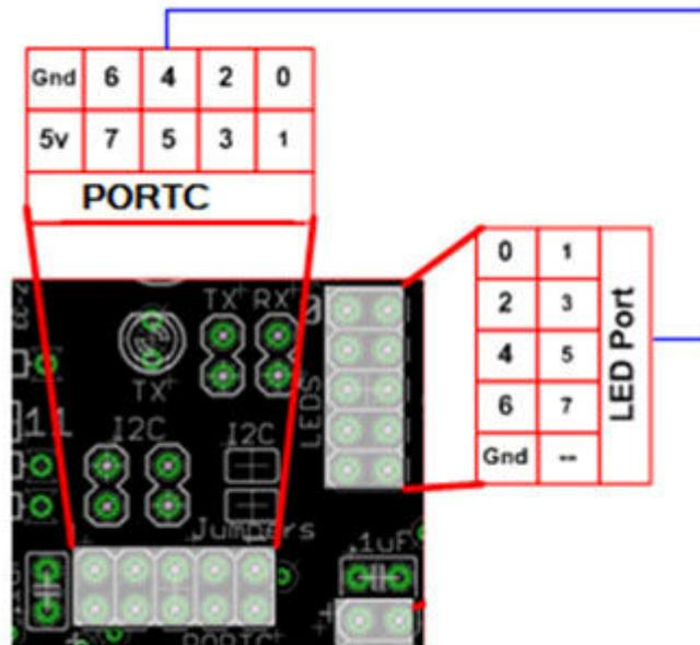
Align the power sides of the ribbon cable, and attach.
