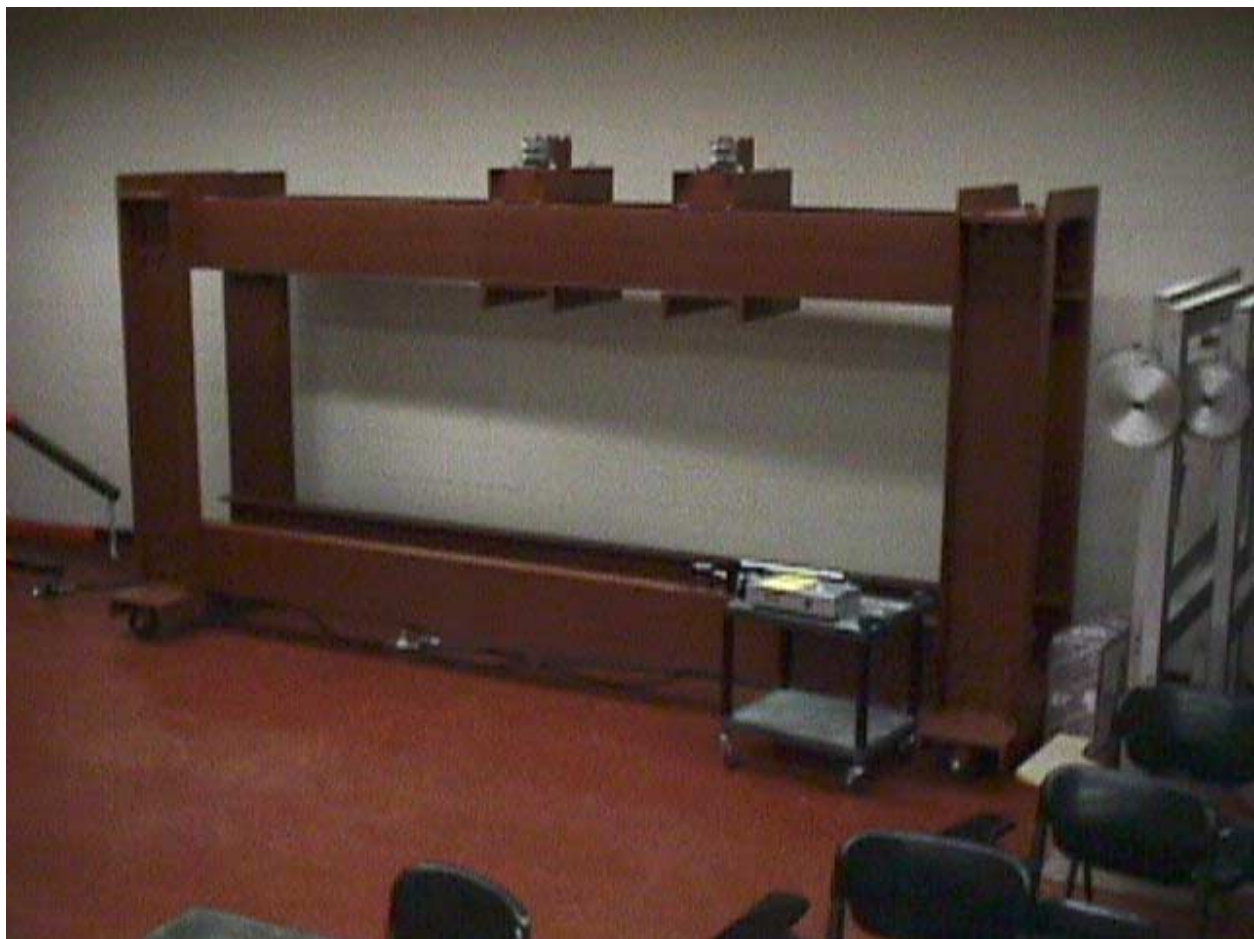
Figure 1. Load frame constructed by the department that was a result of the project work described.
