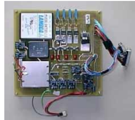
Figure 3. SPECTRE power board before mounting and vibration staking.
