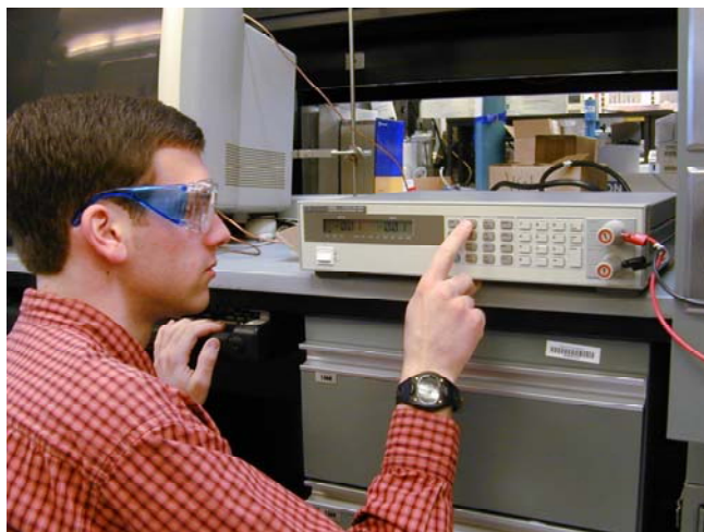
Figure 13: Hewlett Packard 6060B Electronic Load Box
