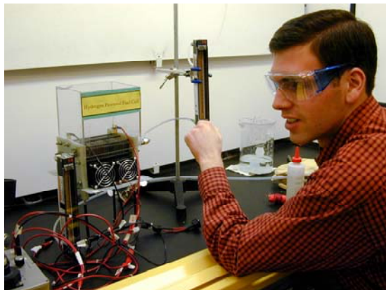
Figure 12: BCS Fuel Cell System
