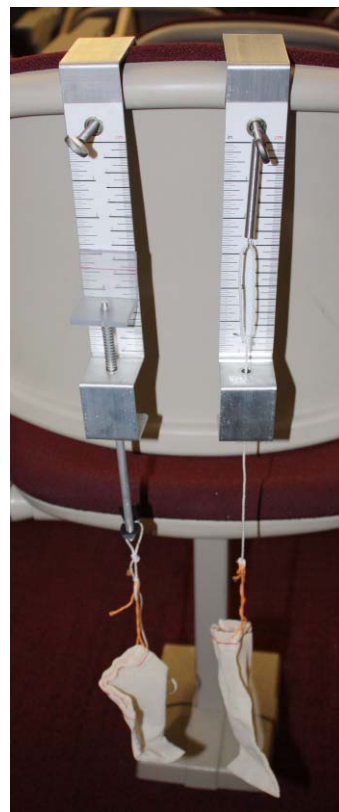
Figure 4: In-class setup for characterizing the spring constants of compression (left) and extension (right) springs using bags of marbles to displace the springs.
