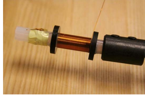
Figure 9: Students use an electric screwdriver to wind copper wire around a plastic tube to make a homemade solenoid for use in the design competition.
