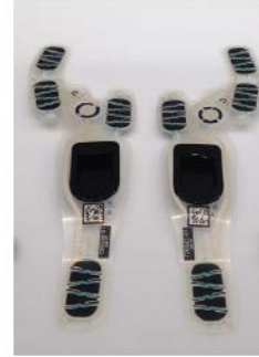
Figure 1. (left) Pack kit: 2 pucks, USB dongle, and receiver module. (right) In-shoe pressure pads: 2 insole-like pads. Reprinted from Nike.com
