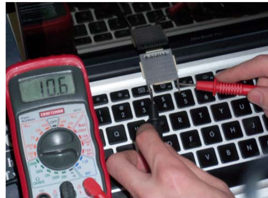
Figure 3: measuring voltage generated using a thermoelectric generator
