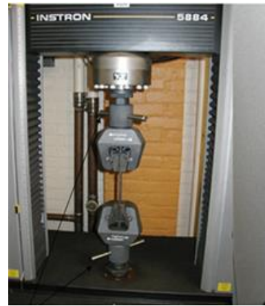
Figure 4. Tensile test with an Instron machine
