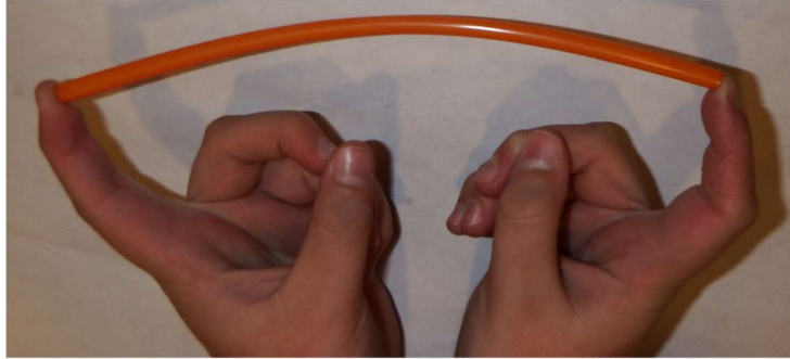
Figure 4: Buckling of a Drinking Straw Column
