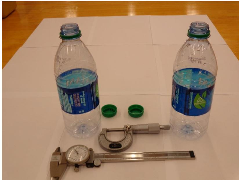
Figure 3: Items for the torsional shear stress and design activity (plastic strip omitted)
