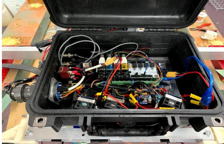
Figure 3: Electronics box containing Central processing unit and electronic speed controllers
