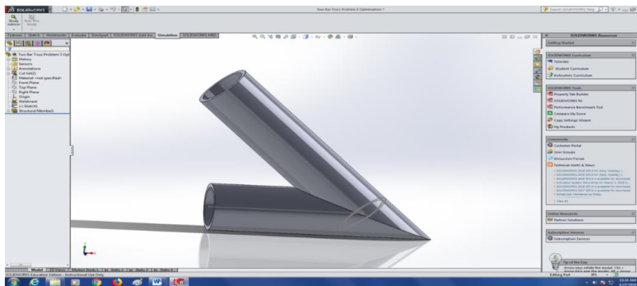
Fig. 11: SolidWorks CAD Model of the Two-Bar Truss with Optimal Values
