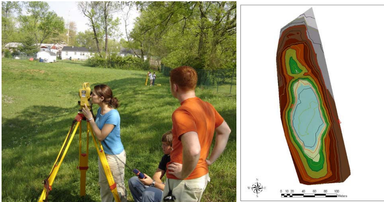
Figure 3. Students performing a topographic survey and the finished product
