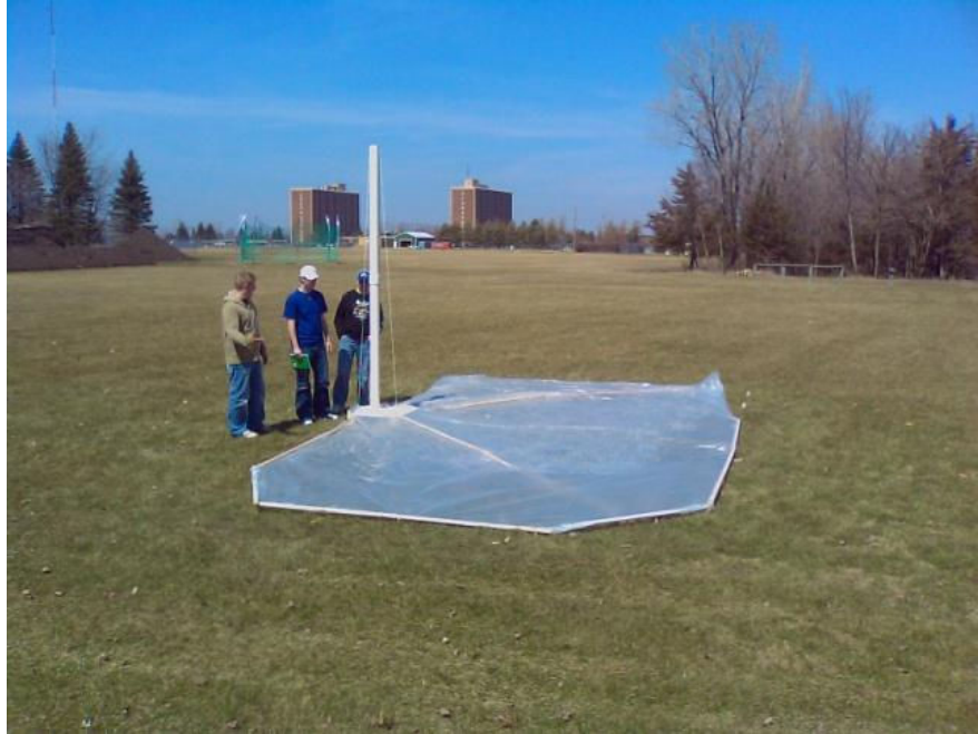
Figure 3: “Three sided” rectangle (25ft by 15ft) collector design.
