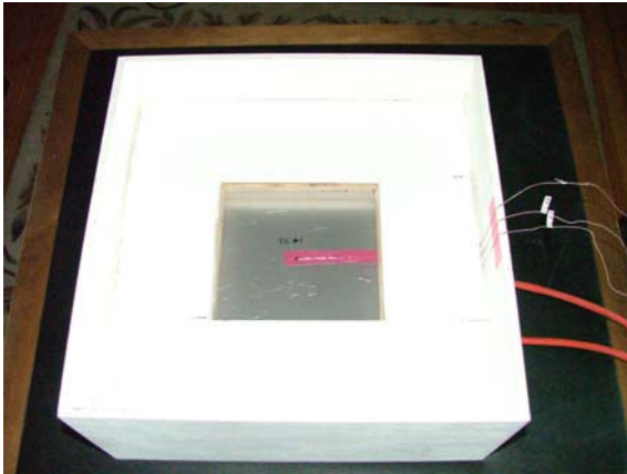
First wall layer, with heat source attached, placed in box. TC # 1 is visible through glass, 2 and 3 are not.
