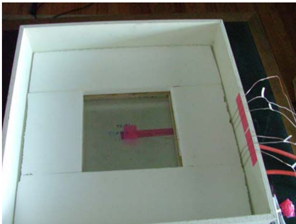
Layer of insulation added over first wall layer.
