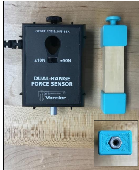
Figure 10. Side by Side Comparison of the Dual Force Sensor and Removable Beam Section's Mounting Capabilities with Supplementary Bottom Section View.
