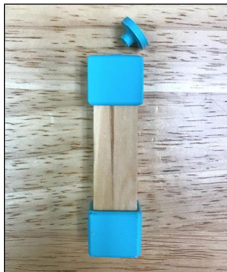
Figure 11. Shear Fracture in Removable Beam Section End Cap
