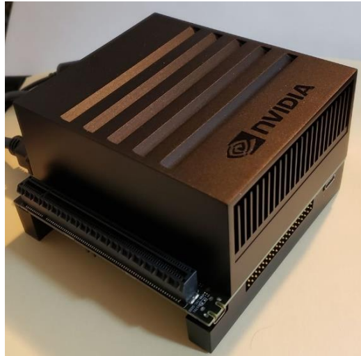
Figure 4. Jetson AGX Xavier Developer Kit by NVIDIA
