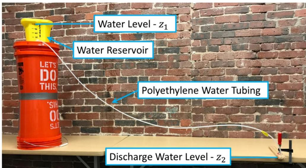
**Figure 2.** Experimental apparatus.
