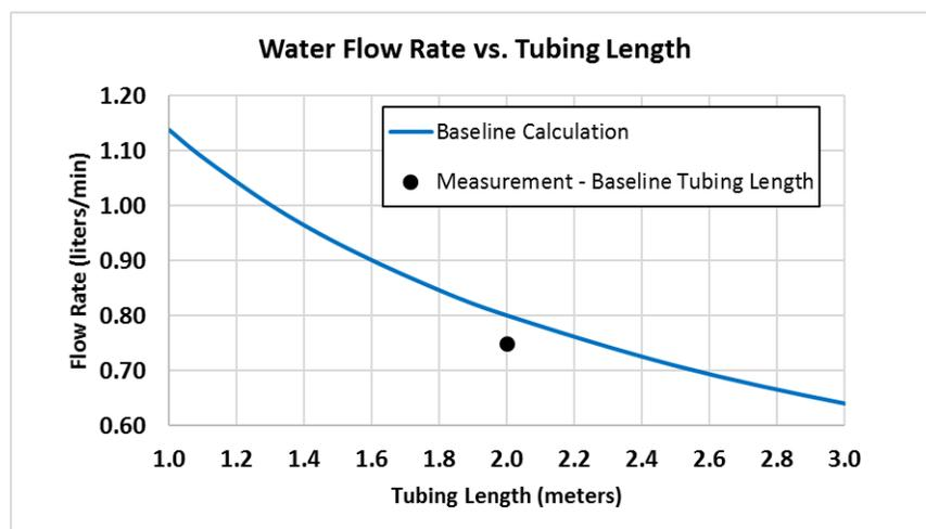
**Figure 5** Calculated variation of flow rates with tubing length and comparison with experimental measurement for 2 meter long tubing.
