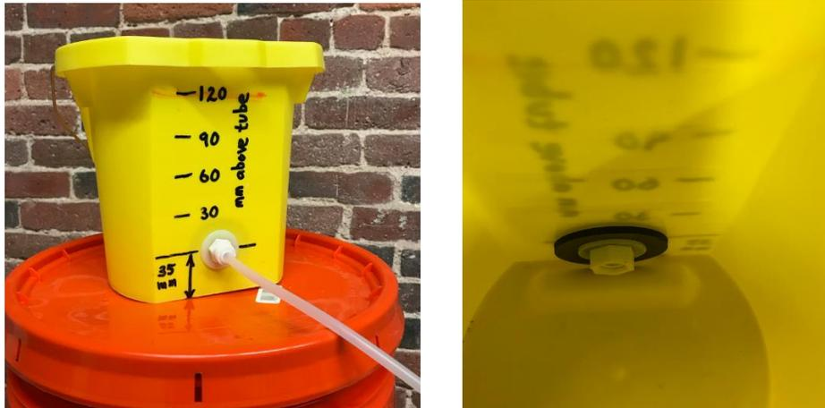
**Figure 3.** Water reservoir showing push-to-attach water tubing fitting. Picture at right shows interior of reservoir with washers used for sealing.
