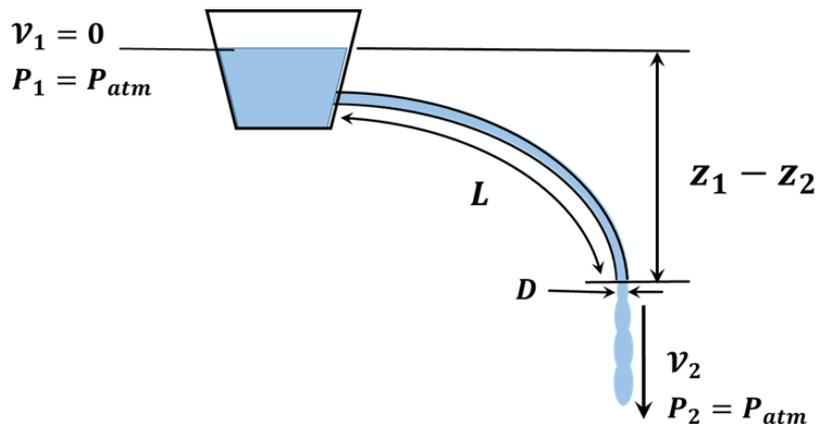
**Figure 1** Schematic of water flow setup showing nomenclature used.
