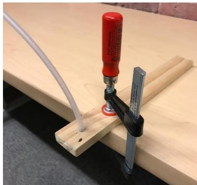
**Figure 4** Clamp and block arrangement for clamping discharge end of tube.
