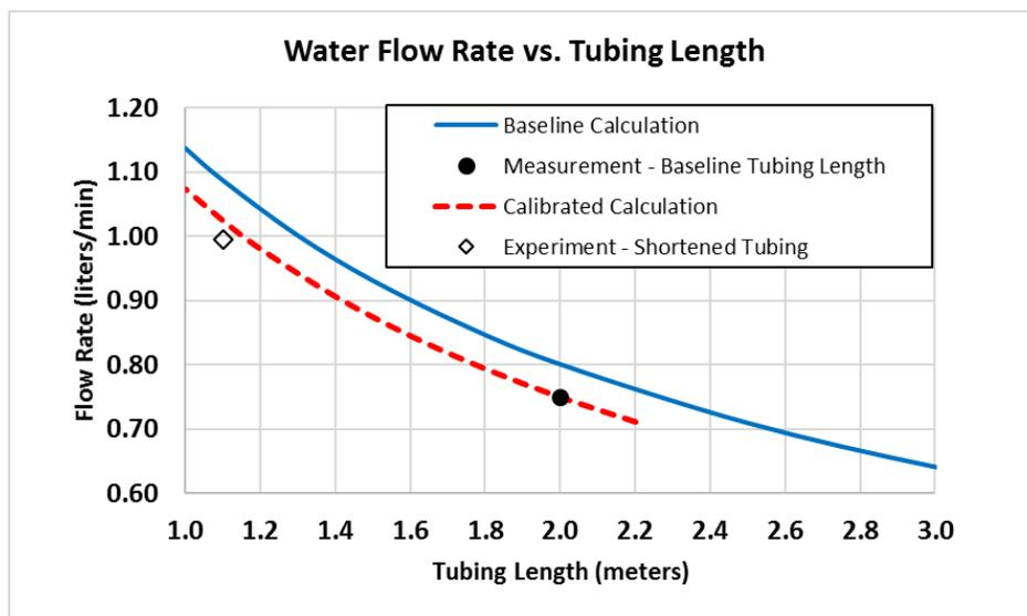
**Figure 6** Flow rate prediction after calibration to baseline experiment, and comparison with measured flow rate for 1.1 meter long tubing.
