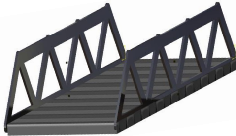
Figure 3: CATIA design of a Warren truss bridge
