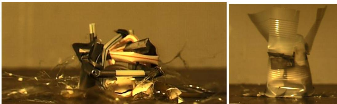
**Figure 2. An egg shattering on impact (left) A Protective Cup Deflecting on impact (right)**
