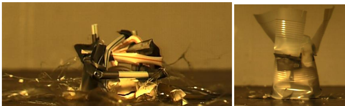
Figure 2. An egg shattering on impact (left) A Protective Cup Deflecting on impact (right)
