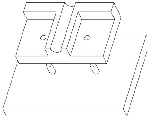
Figure 1. A part modeling and GD&T scheme based on the hole centers being the secondary datum.
