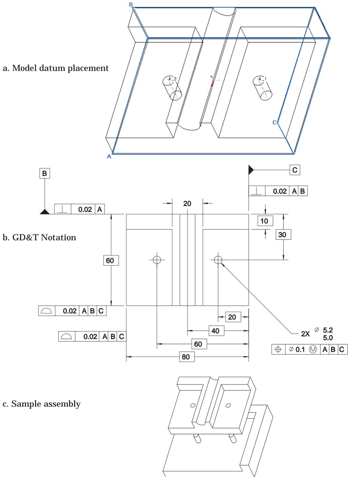
Figure 2. A part modeling and GD&T scheme based on the part edges being the secondary and tertiary datums.
