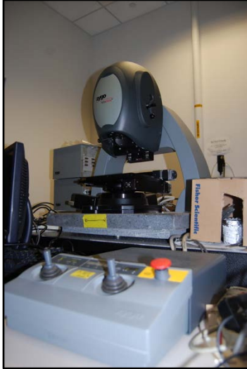
Figure 6: White Light Interferometer Surface Profiler (Zygo NewView 6000)
