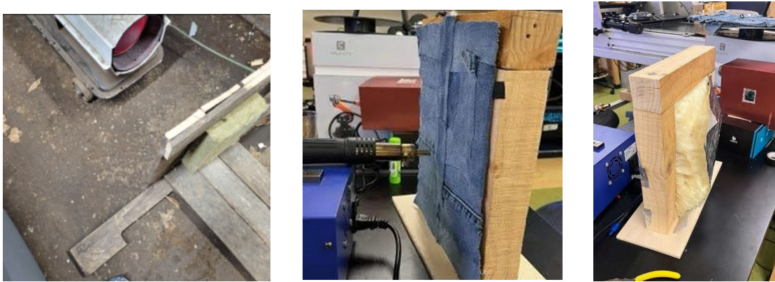
Figure 8: Spring 2023 experimental testing of Rockwool (left), denim/feather combination (center), and spray foam (right) insulation.
