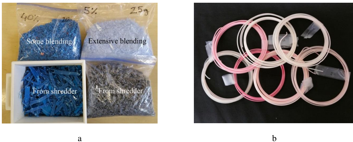
Figure 4. Recycled plastic: a) shredded and mixed PLA b) filament of various mixture ratios
