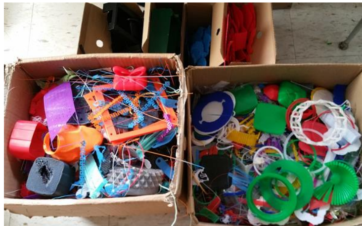
Figure 2. 3D printing scrap material (failed prints, support material, bad designs)
