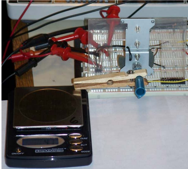
Figure 10 Synchronous motor output power measurement
