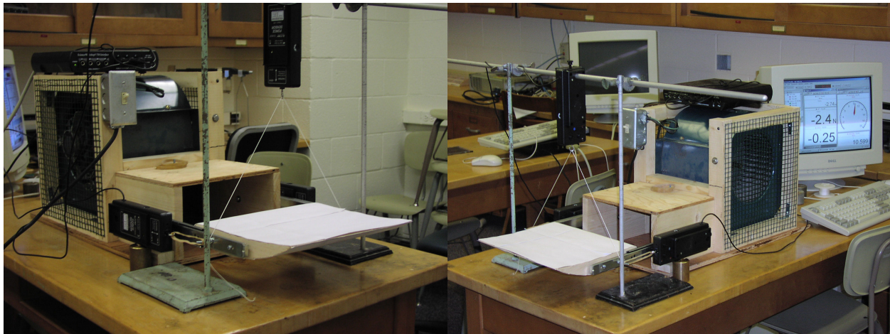
Figure 3: Test stand for the airfoil experiment. See the appendix for a brief description of the set-up. (These figures are 2M resolution and can be enlarged for better viewing).
